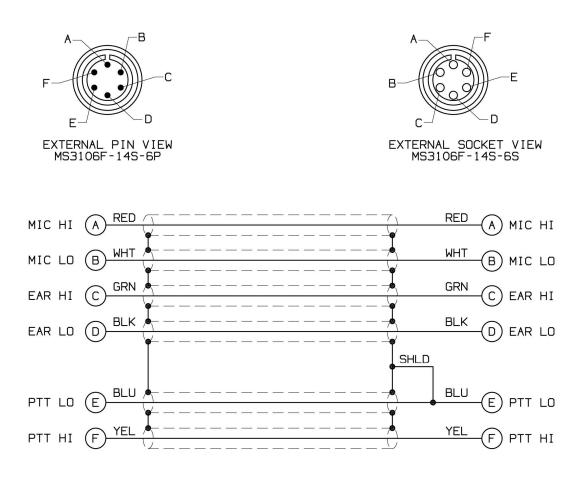
Figure 1. Model C3821-05 Radio Interface Cord Schematic Diagram.
