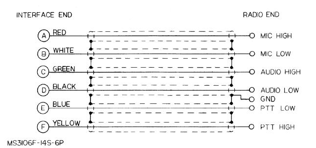
Figure 1. Model C3821 Radio Interface Cord Schematic Diagram.
